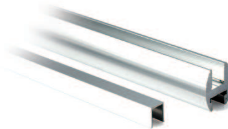
KC10 Length: 2.49 m Includes: Header, u-channel cover for open channel For 8 - 10 mm glass Finishes: CR, PN and BK
